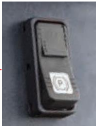
Parking Brake Switch With auto parking function when the operator is not in the seat
