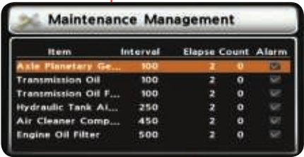
Maintenance Management Display
