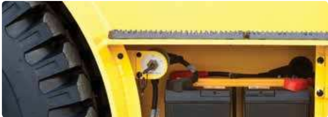
Master Switch A master switch disconnects the battery power to protect the electrical system from excess electrical drainage. (optional)
